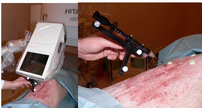
Fig. 14. Optical tracking device for measuring spatial location of a surgical instrument.
