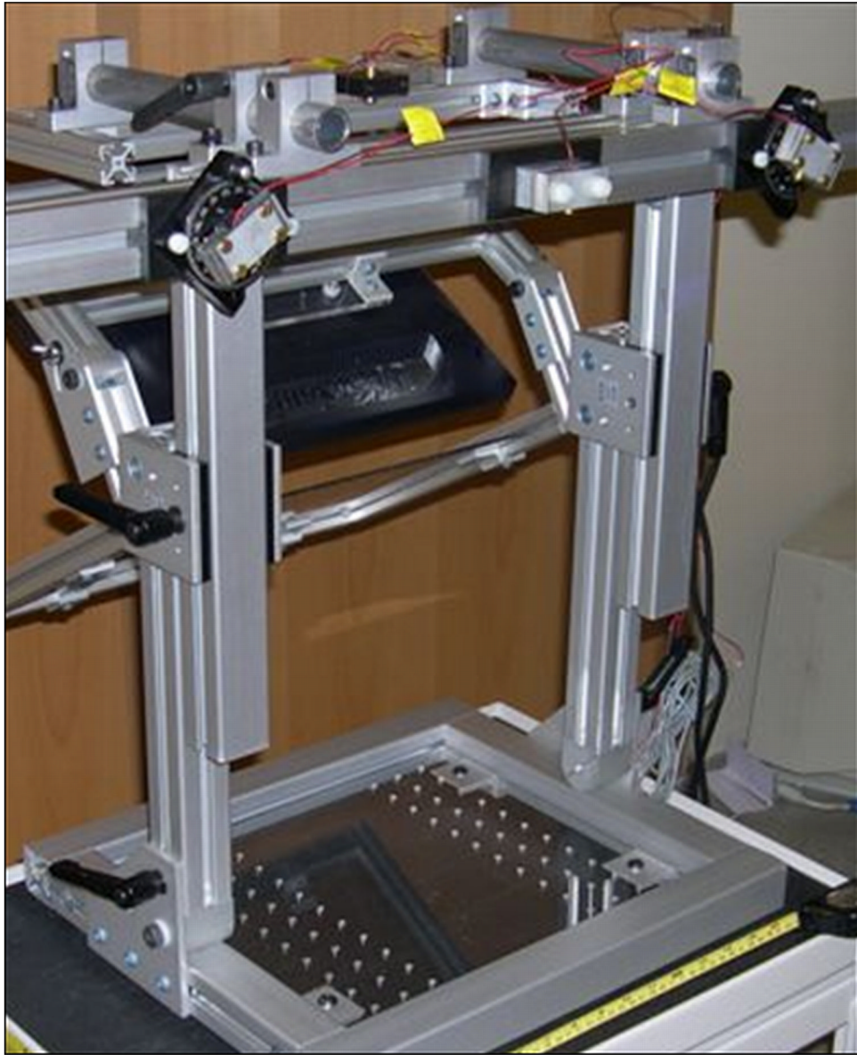
Figure 3. The Perk Station – actual prototype; image overlay (left) and biplane laser overlay (right)
