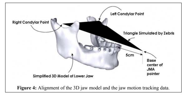
that is attached to the ultrasonic emitter array. The 3D mandibular model is then aligned in space as shown in Figure 4 such that the condylar points coincide with the corresponding points on the triangle and the base center of the JMA T-attachment is at a distance of 5cm from the jig.
