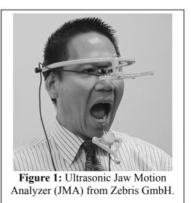
head frame secured to the patient's head. The spatial coordinates of the two condylar points and an infraorbital point are pre-selected by the user to define a plane. Movements of at least three points relative to this plane during jaw motions are saved in an ASCII file. The three points are the two condylar points and the base center of the T-attachment pointer attached to the jig.
