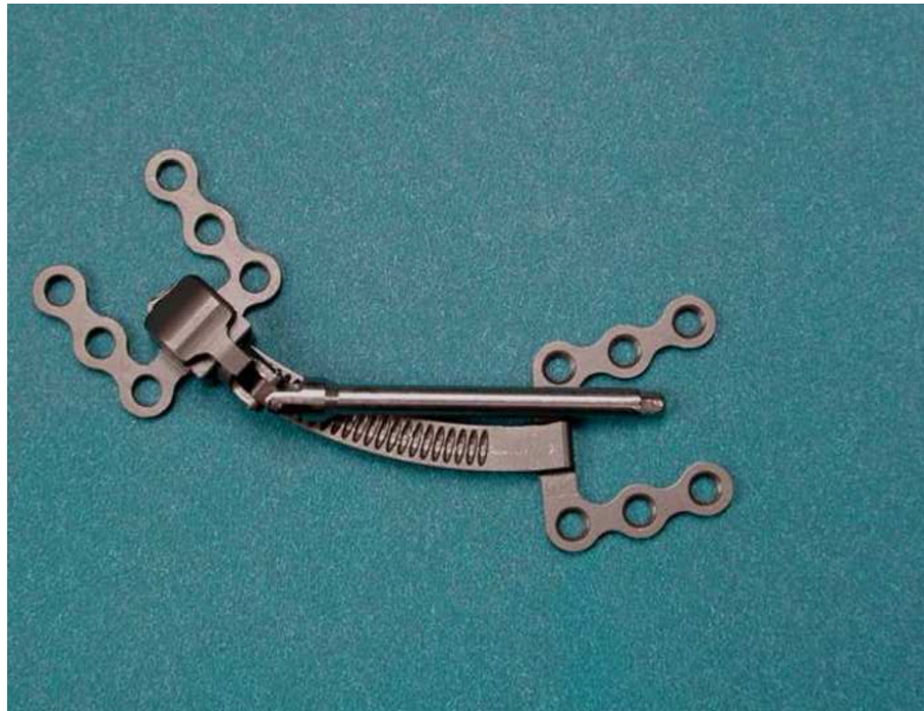
Figure 1. (A) Semiburied, curvilinear distraction device (Synthes CMF, West Chester, PA) for left ramus: Radius of curvature 5cm, elongation parameter 25mm (Note the worm gear housing and the curved track along which distractor and distal mandible move). (B) Device fully activated.
