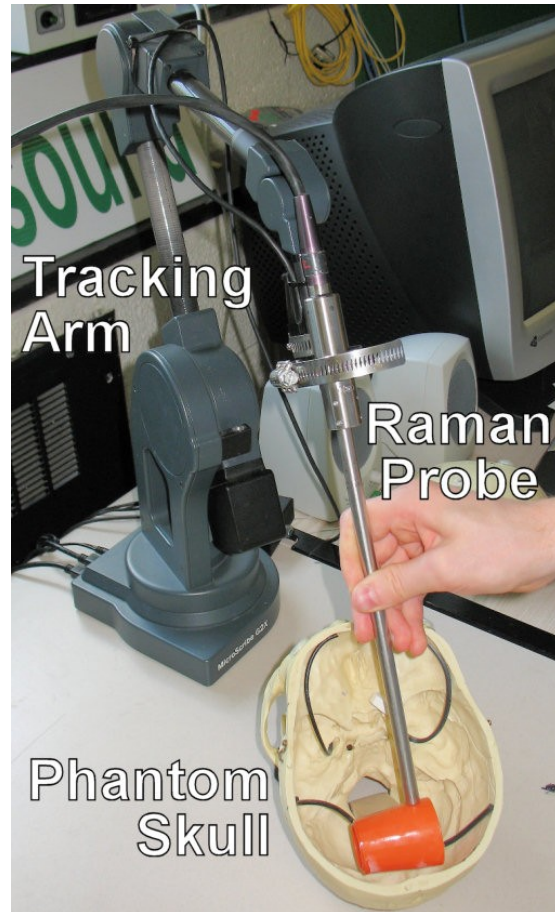
Figure 2: The Raman probe, attached to the end of the tracking arm, is used to scan a plastic cup and other objects within the phantom skull
