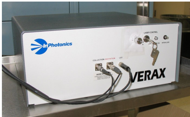
Figure 3: The Verax portable Raman spectrometer with an attached fiber optic probe
